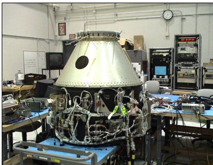
Figure 111-1: Electro-mechanical fit check and a separation test
