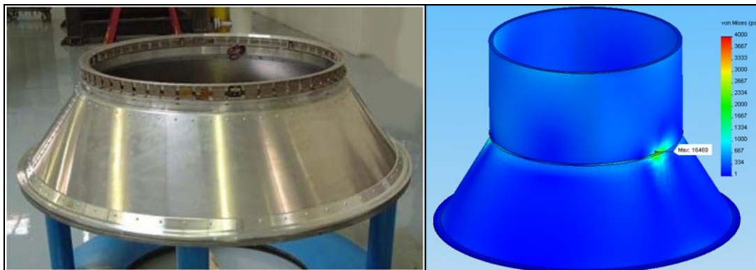
Figure 4-11: An MLB attached to a launch vehicle cone and CAD model showing resulting stress peaking that occurs when adjoining two warped surfaces
