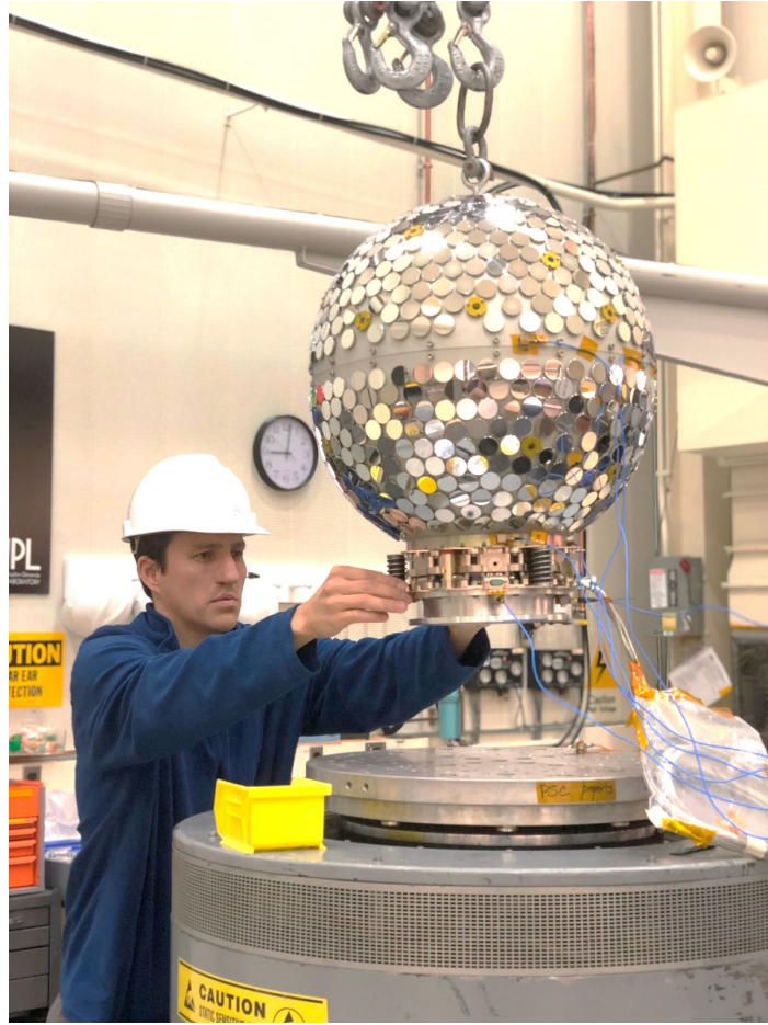
Figure 2-2: An ALB attached to Starshine-4 during a pre-flight vibration test
