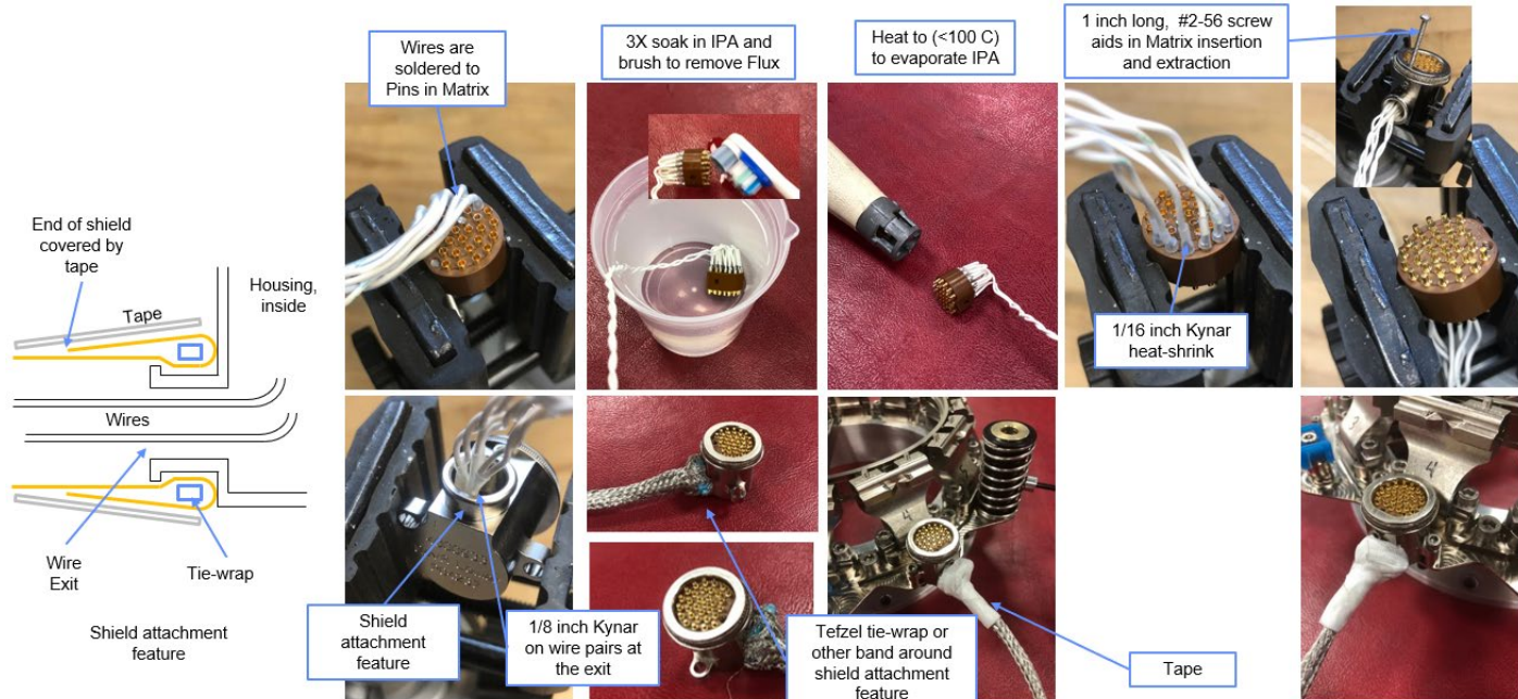
Figure 144-5: Wiring of Separation Connector
