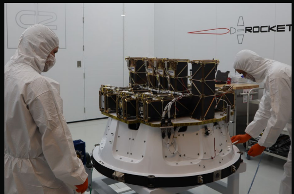
◉ 'ELANA-19' PAYLOAD INTEGRATION ONTO THE KICK STAGE | 2018
