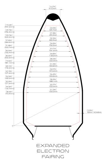
Figure 17 Expanded Electron Fairing
