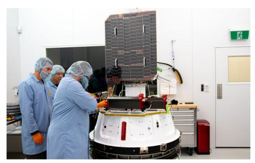
Figure 42 Flight 7 'Make It Rain' Payloads Intergrated With Rocket Lab's Kick Stage
