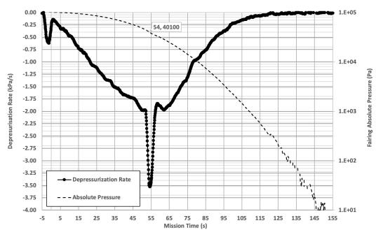
Figure 26 Electron Typical Fairing Venting Environment
