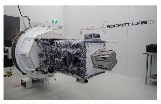
Figure 40 DARPA Spacecraft Intergrated with Rocket Lab's Kick Stage
