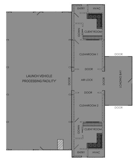
Figure 44 The layout of the Payload Processing Facility at LC-1
