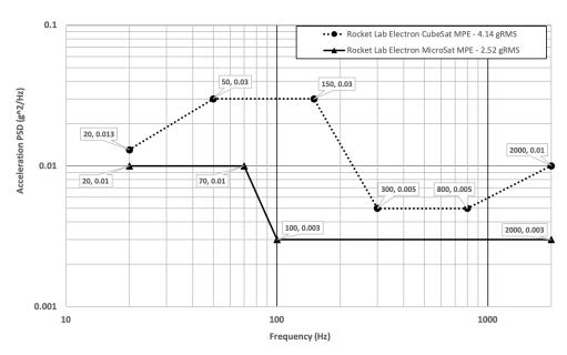
Figure 25 Electron Random Vibration MPE
