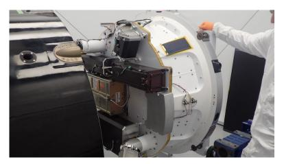
Figure 7 Rocket Lab's Kick Stage being intergrated with the fairing
