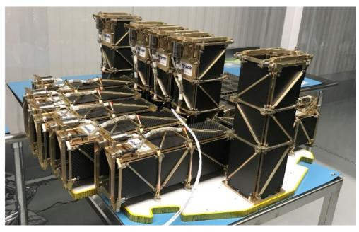
Figure 19 Rocket Lab payload plate, payload configuration for NASA ELaNa-19 mission
