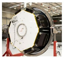
Figure 10 Photon LEO configuration (payload plate view)
