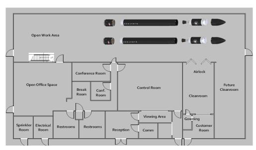
Figure 46 The layout of the Payload Processing Facility at LC-2
