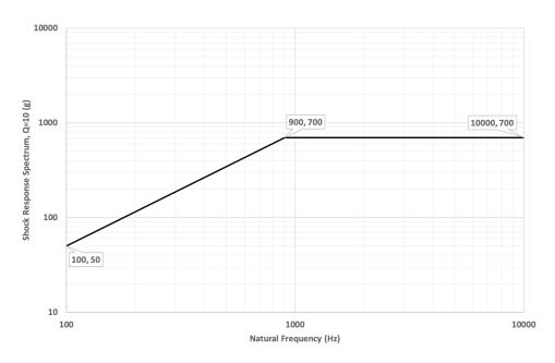
Figure 23 Electron Shock MPE
