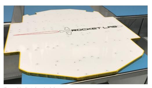
Figure 18 Rocket Lab payload plate
