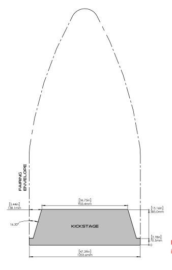
Figure 8 Rocket Lab's Kick Stage inside the fairing envelope
