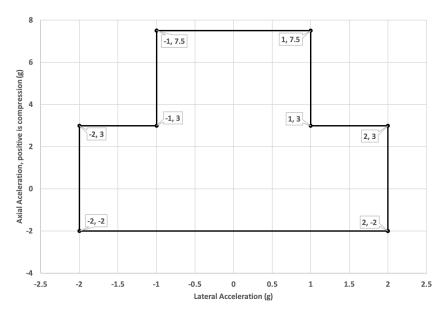
Figure 22 Electron Acceleration MPE
