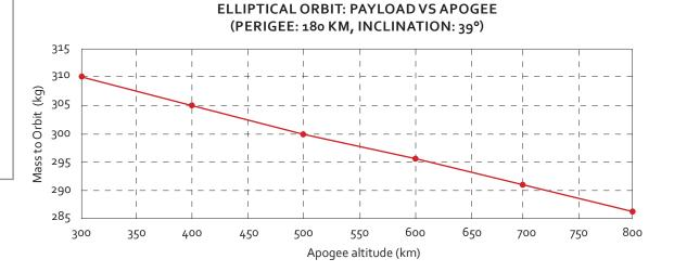
Figure 13 Performance to a 180 km Perigee at 39° Inclination Elliptical Orbit
