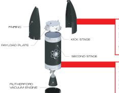
At the top of the Electron rocket is the fairing, or nose cone. These two structures protect the satellite inside it when Electron is flying through Earth's atmosphere on the way to space. The fairing is jettisoned before the payload is deployed. Inside the fairing sits the satellite. It is
