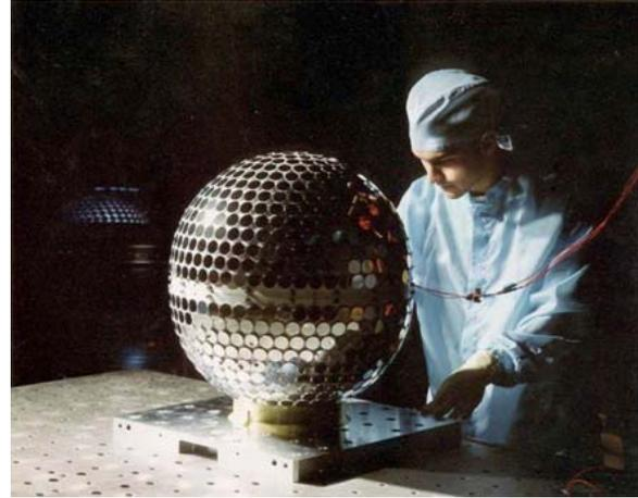
**Figure 5: Starshine 1 on NRL Vibration Table**
