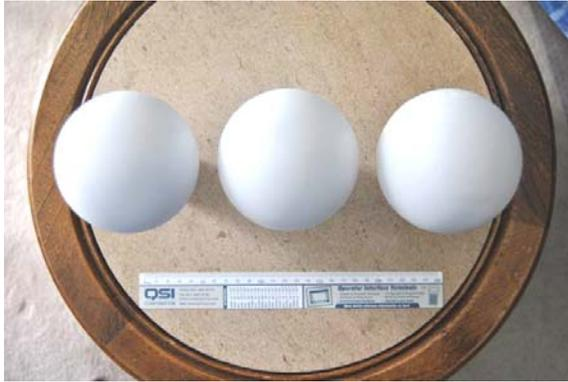
**Figure 1: Three 10-cm Diameter Hollow Aluminum White Painted POPACS**
