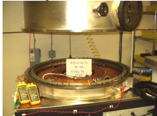
**Figure 15 Thermal Vacuum chamber with 38 inch Lightband**
