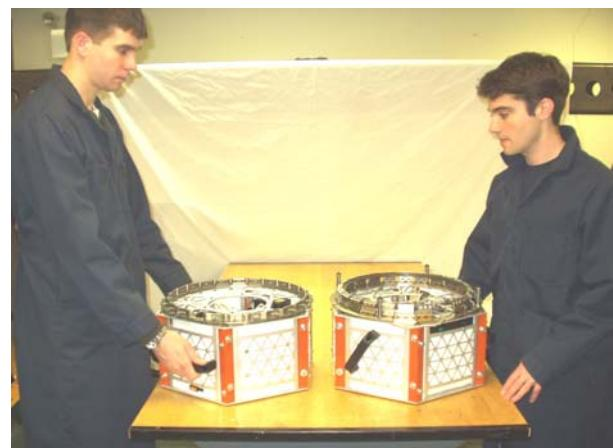
Figure 5 The satellites are removed from their crates, the Lightband halves have previously been integrated to adjoining vehicles
