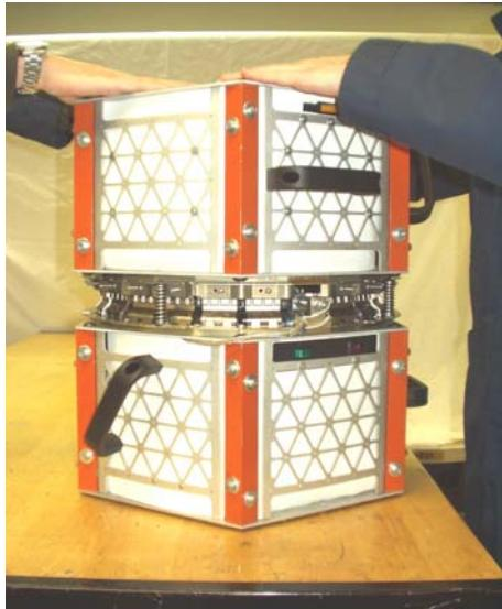
**Figure 7** The satellites are joined using integral clocking and alignment features
