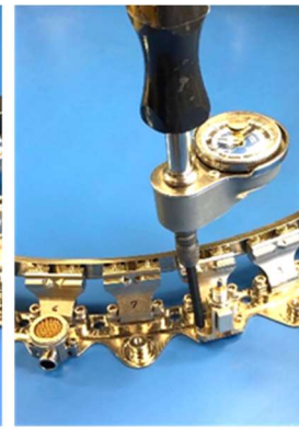
Tighten screws with Torque Wrench
