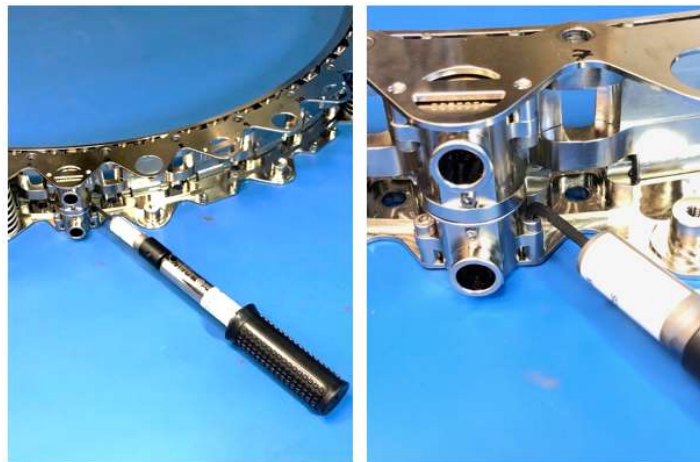
Figure 11-7: Separation Connector attachment torque
