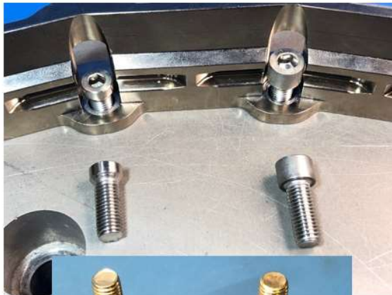
Figure 9-2: Fasteners and torques for adjoining structures
