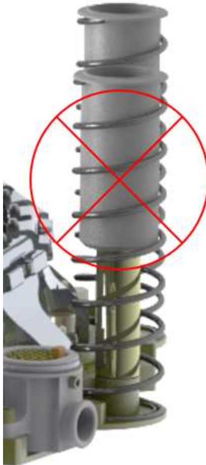
Figure 7-4: Do not use Springs to rotate ALB
