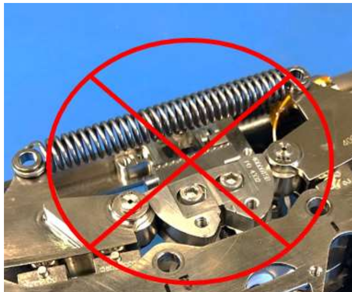
Figure 7-2: Avoid Initiation area when handling
