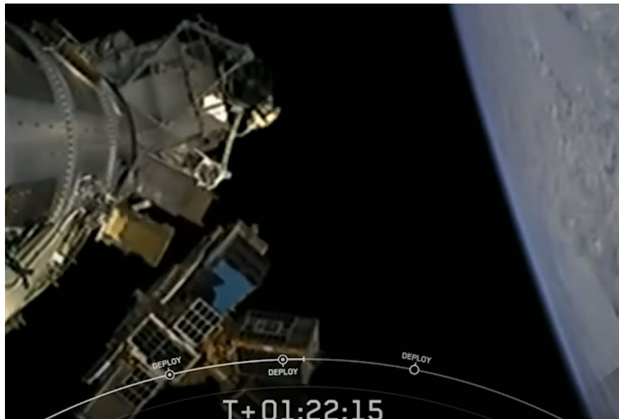
Figure 2-3: Two ALB 24 Separate FX-2 and LTE-1 from SpaceX's Transporter-2 using ALB 24
