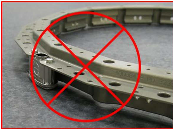
Figure 6-8: Do not allow Upper Ring accessories to contact anything
