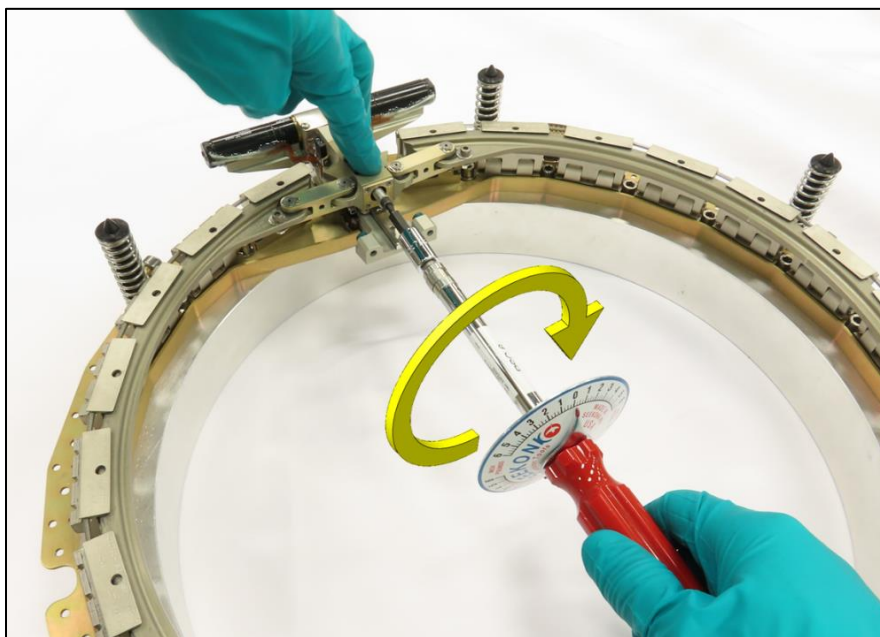
Figure 8-3: Rotating ball screw to allow Sliding Tube travel
