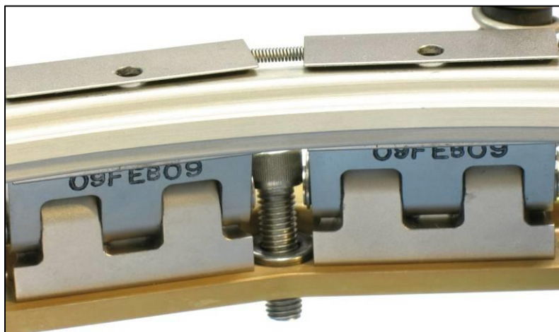
Figure 12-2: Removing a SHC screw from the Lower Ring, inner view
