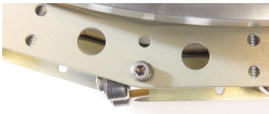
Figure 18-3: Visually aligned LCT pair
