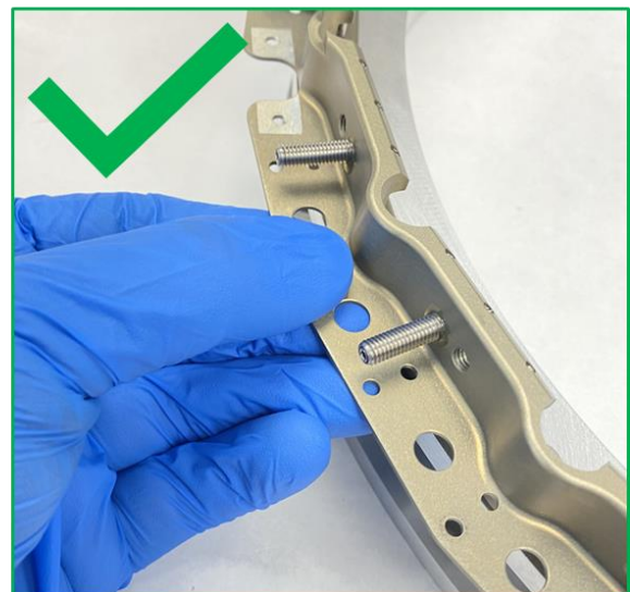
Figure 6-9: Uses flanges to handle the Lightband
