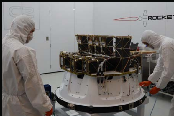
◉ 'ELANA-19' PAYLOAD INTEGRATION ON THE KICK STAGE | 2018
