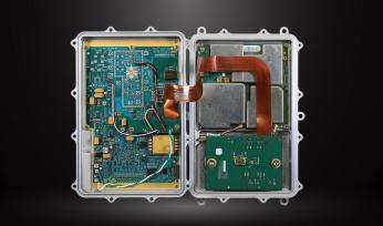
The Frontier-X by Rocket Lab is a high-speed, X-band, software-defined telemetry, tracking, and control (TT&C) X-band radio designed for both near Earth and deep space missions.
