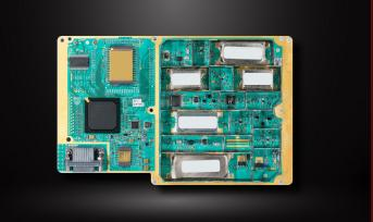
The Frontier-S by Rocket Lab is a single board, software-defined telemetry, tracking, and command (TT&C) S-band radio designed for both near Earth and deep space missions.
