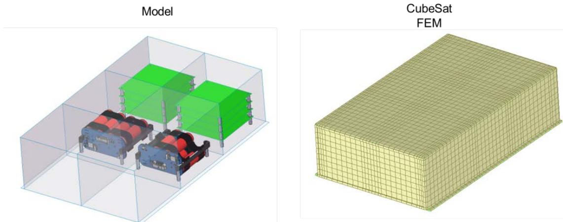
Figure 2-3: Satellite model and FEM
