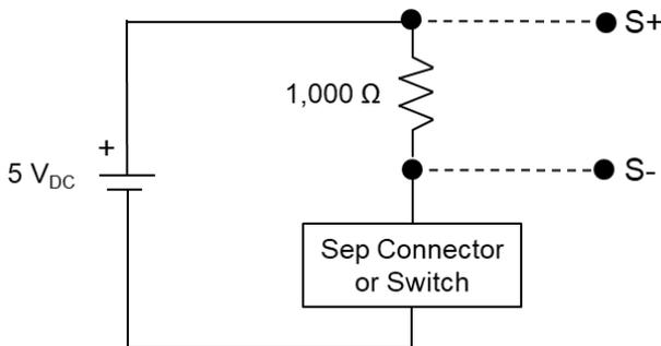
Figure 7-3: Measurement circuit
