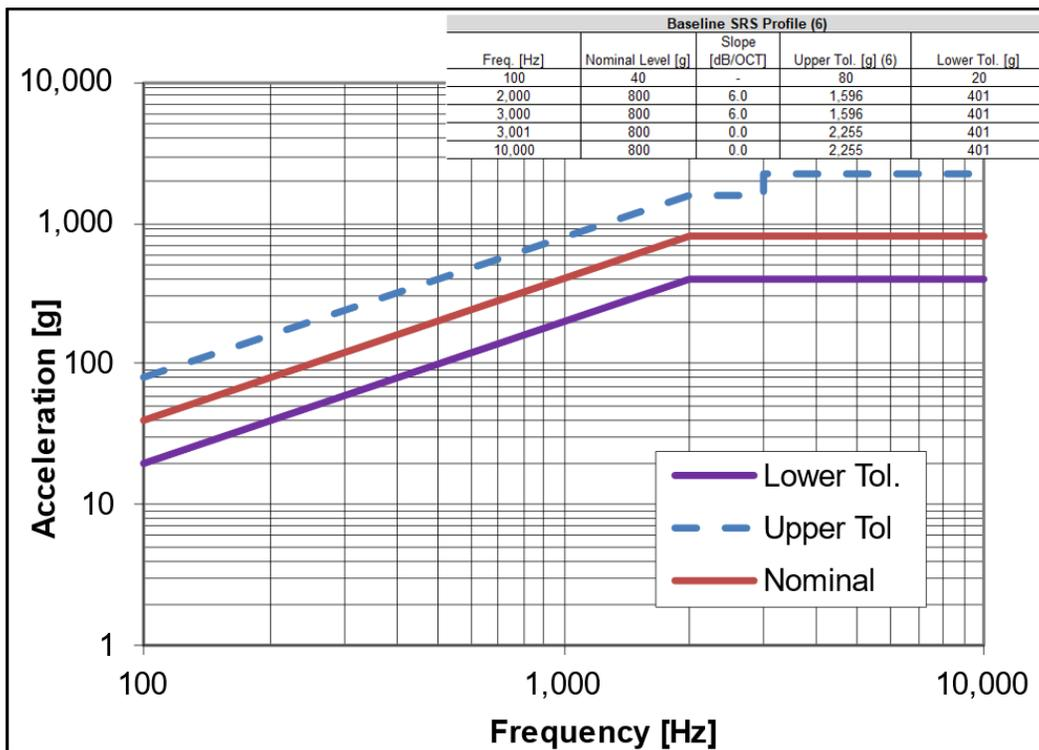
Figure 9-3: ASD applied shock specification
