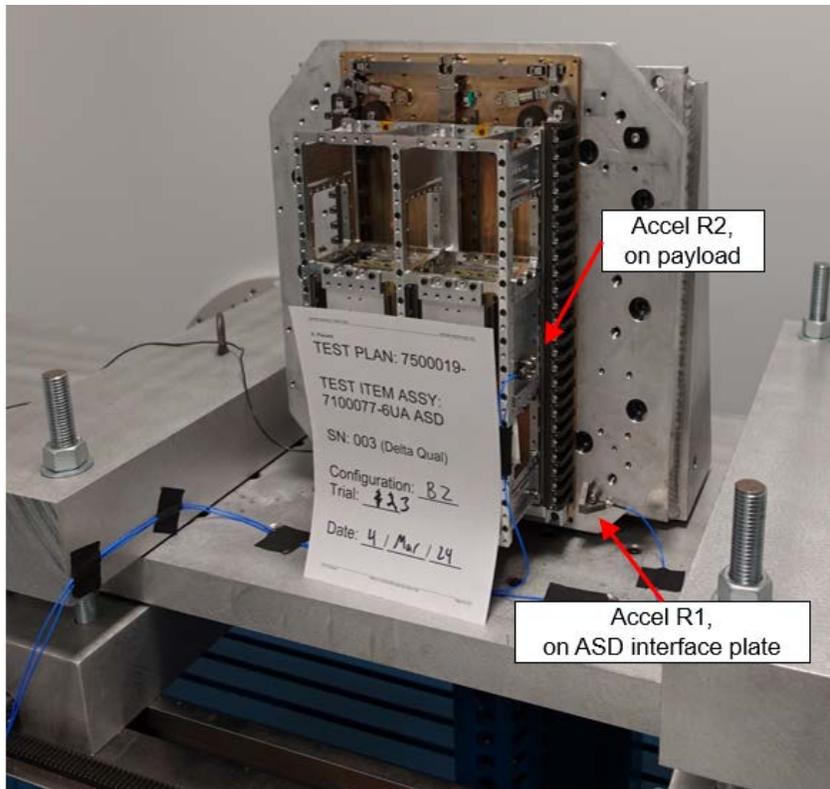
Figure 9-4: Qualification applied shock test setup, 6U, Z axis, no walls
