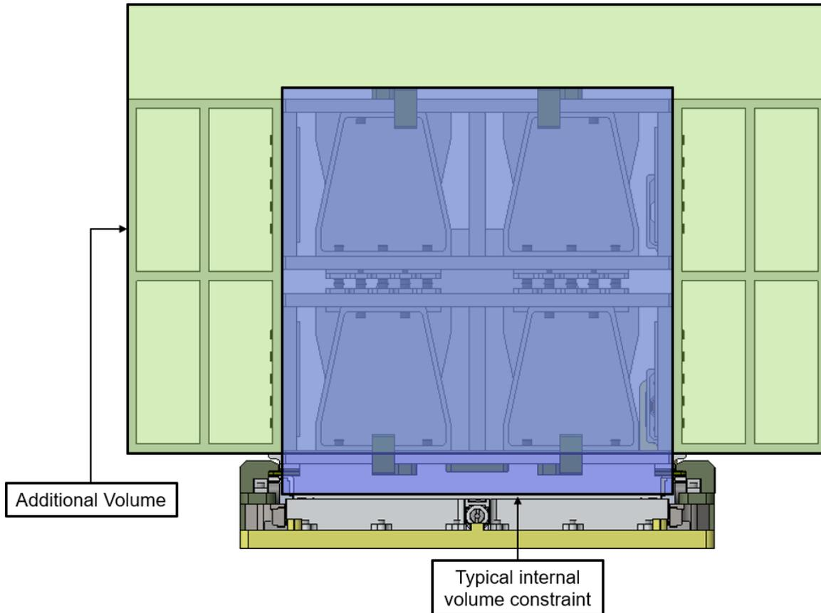
Figure 15-2: Example of extended XY payload volume
