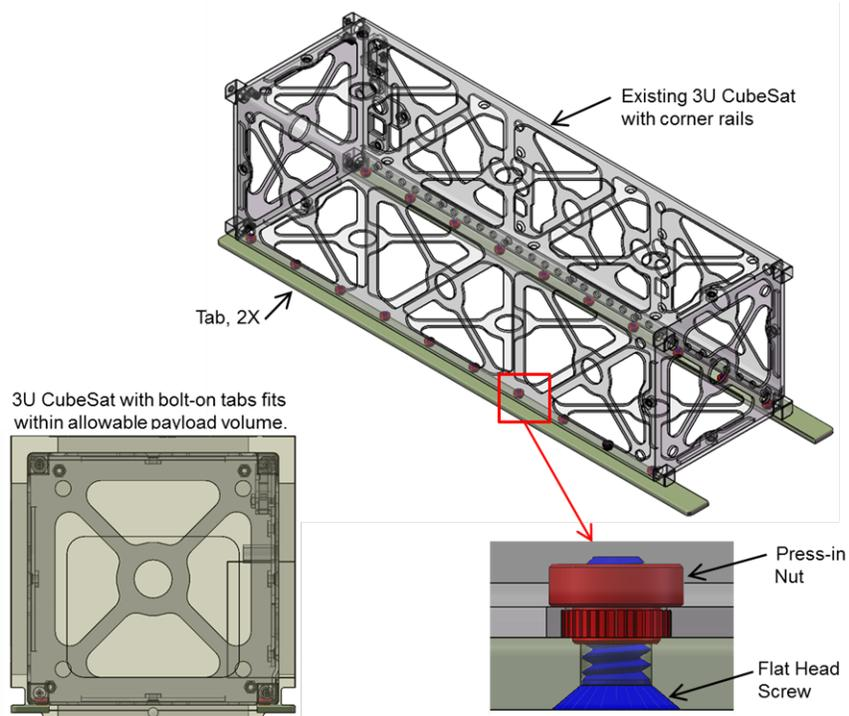
**Figure 15-6: CubeSat with bolt-on tabs**
