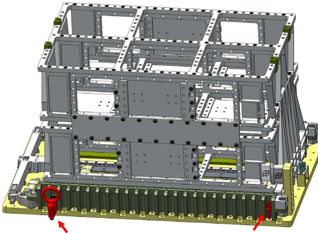
Figure 23-1: 12U ASD with various examples of eyebolts for lifting
