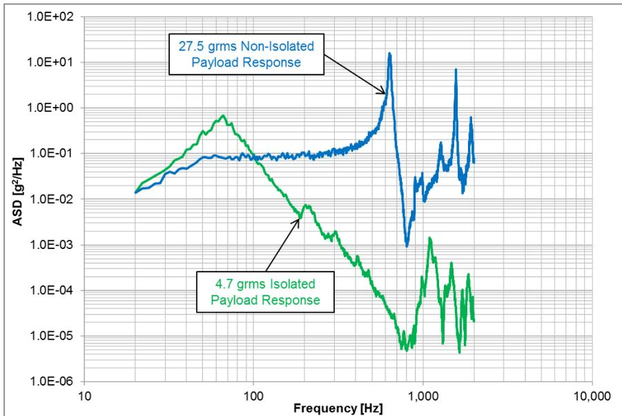
Figure 14-1: Isolation system benefits during random vibration testing
