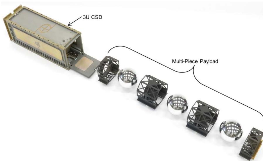
Figure 15-4: A single CSD/ASD can dispense multiple payloads (ref. 2, 6)
