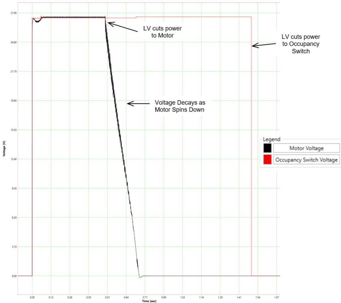
Figure 8-1: Example initiation voltage profile
