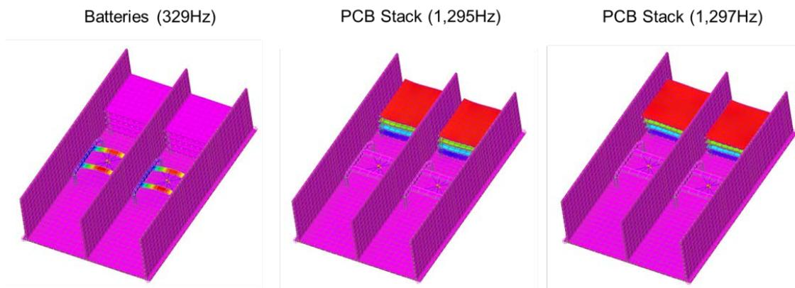
Figure 2-4: Normal modes analysis of satellite elements
