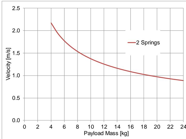
Figure 10-1: Estimated payload ejection velocity
