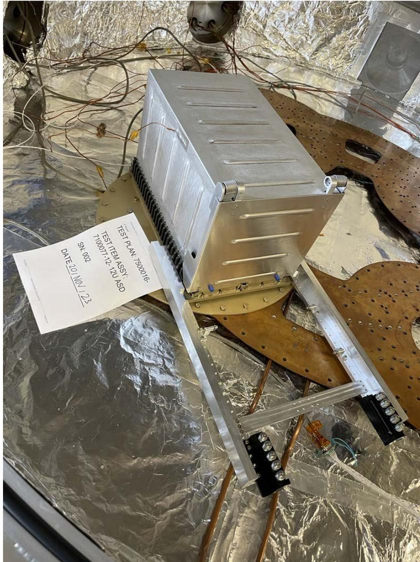
Figure 9-1: TVAC testing an ASD in one of PSC-RL's chambers. Conveyors allow complete payload dispensing (see Section 16).
