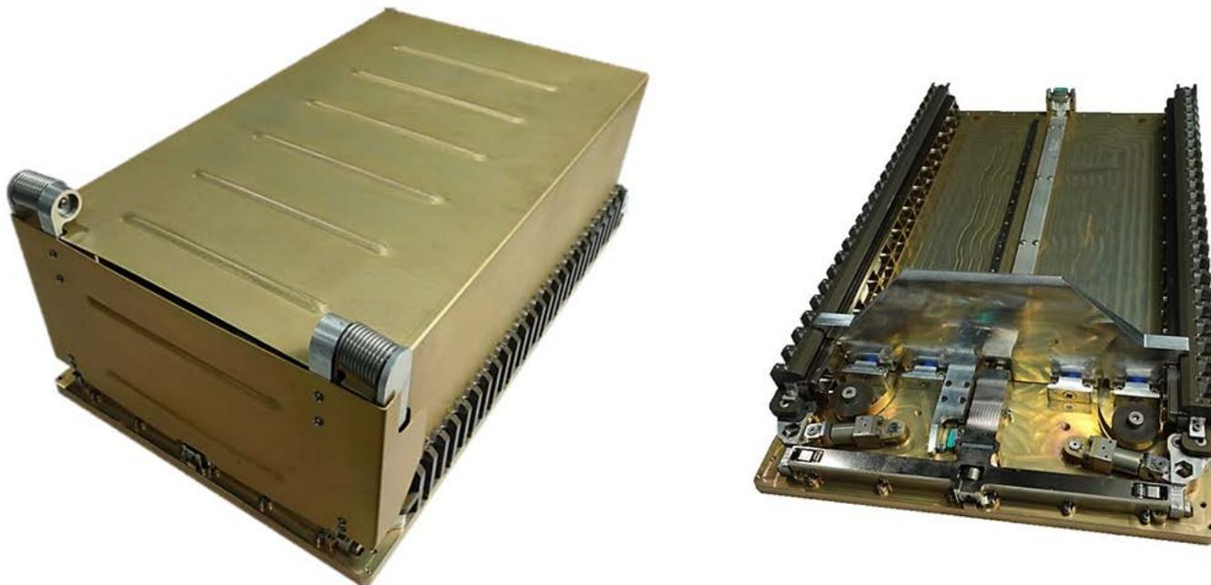
Figure 1-1: ASD with and without walls (6U shown)
