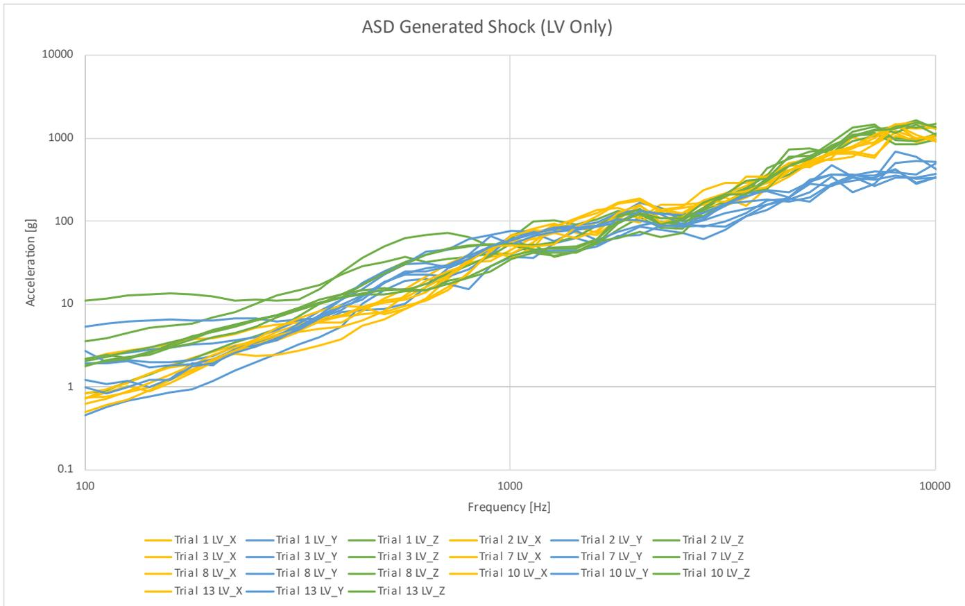
Figure 9-9: Shock measured on the aluminum plate
