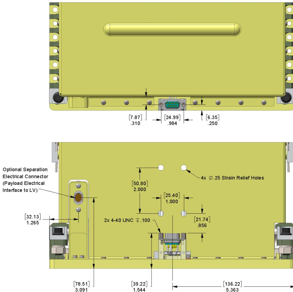
Figure 6-1: Launch vehicle electrical interface
