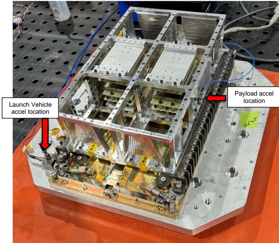
Figure 9-6: Generated shock, light payload test setup
