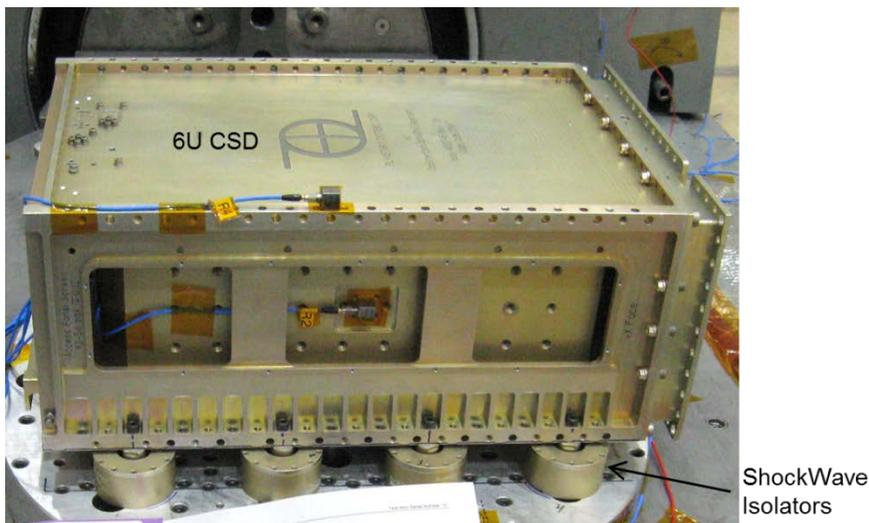
Figure 14-2: 6U CSD vibration test with Moog CSA ShockWave isolators
