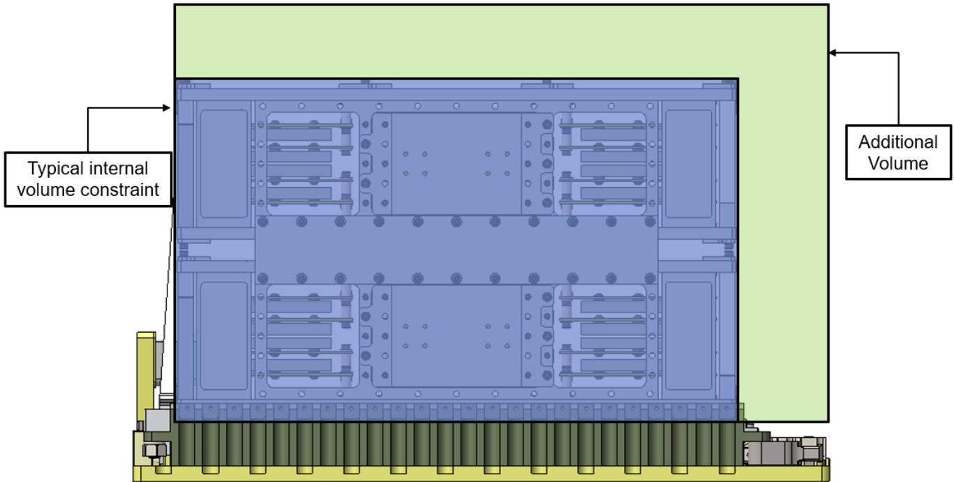
Figure 15-3: Example of extended YZ payload volume
