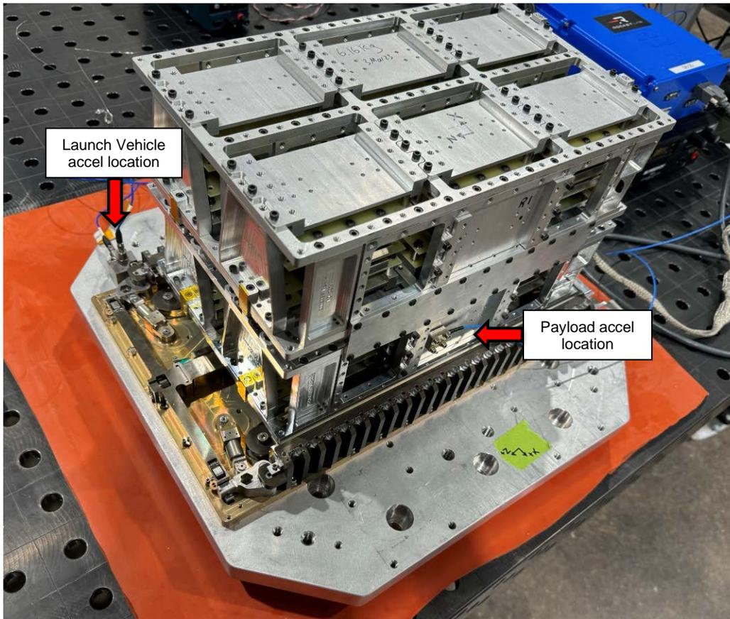
Figure 9-7: Generated shock, heavy payload test setup
