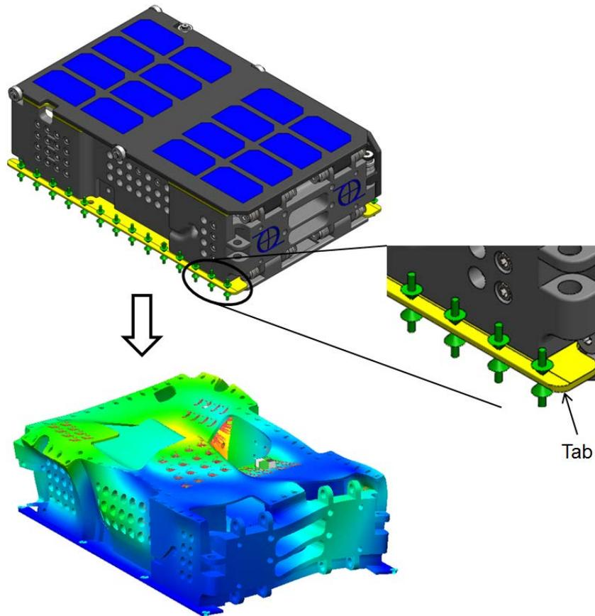
Figure 2-1: 6U payload predicted dynamic response
