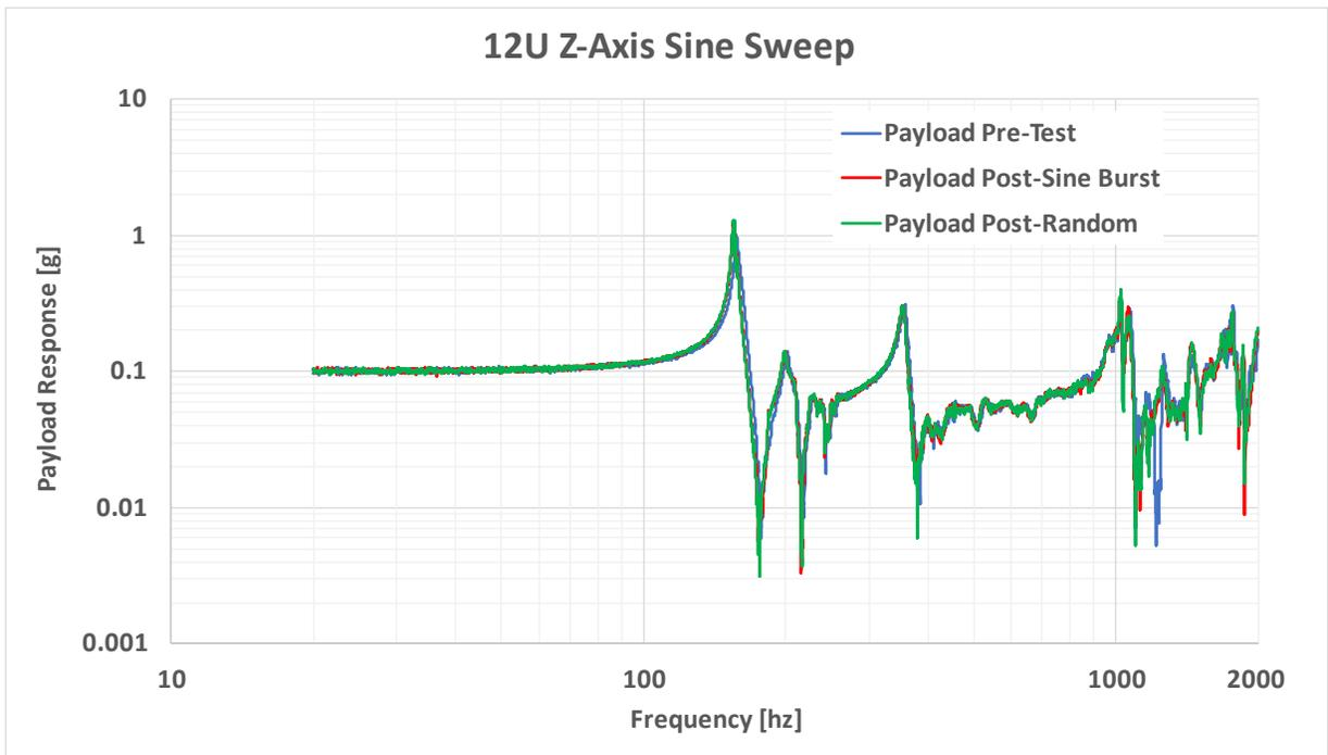
Figure 2-7: Actual payload sine sweeps
