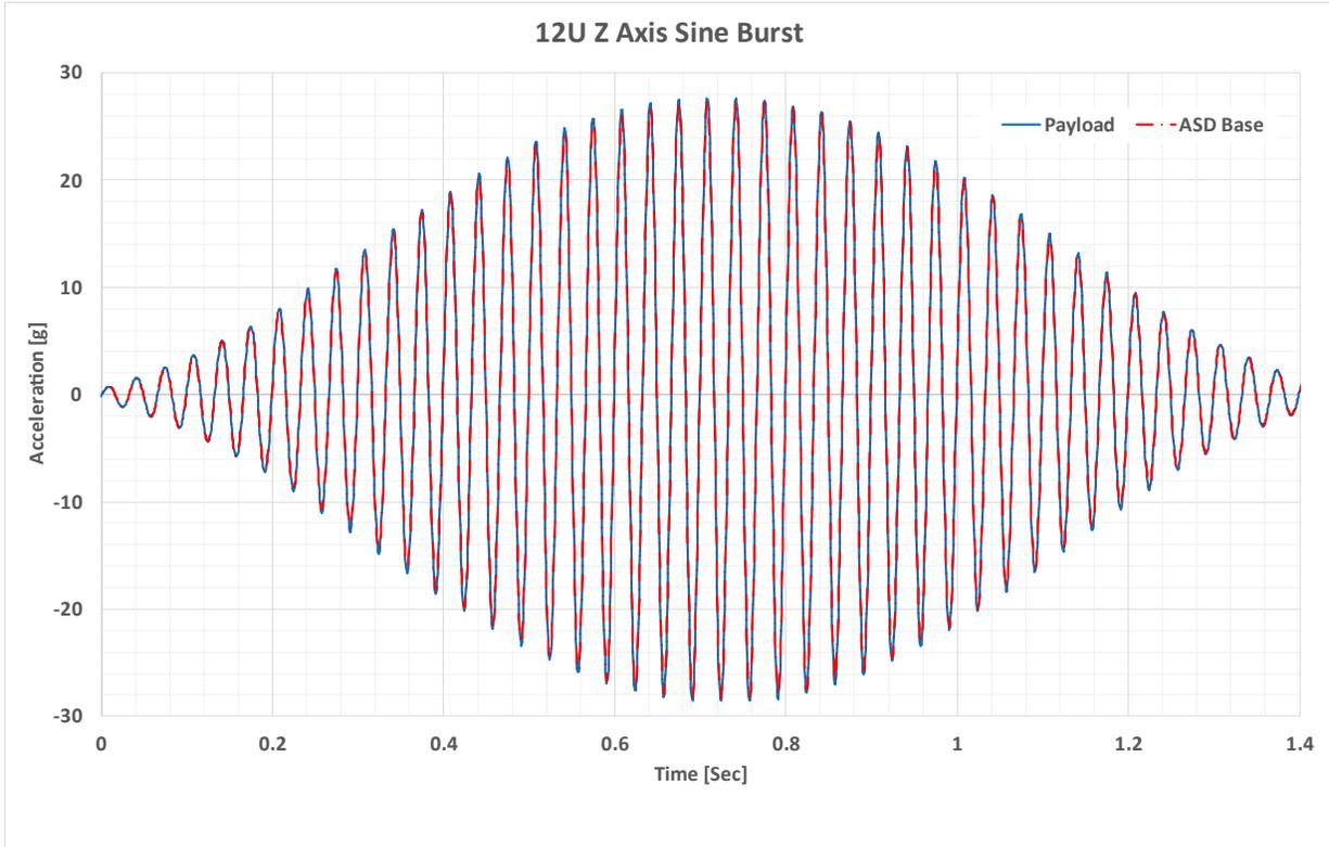
Figure 2-6: Actual payload and ASD response during a sine burst test
