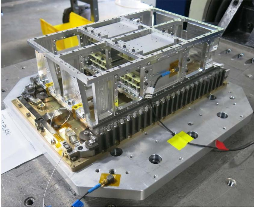
Figure 9-2: Typical ASD acceptance random vibration test setup
