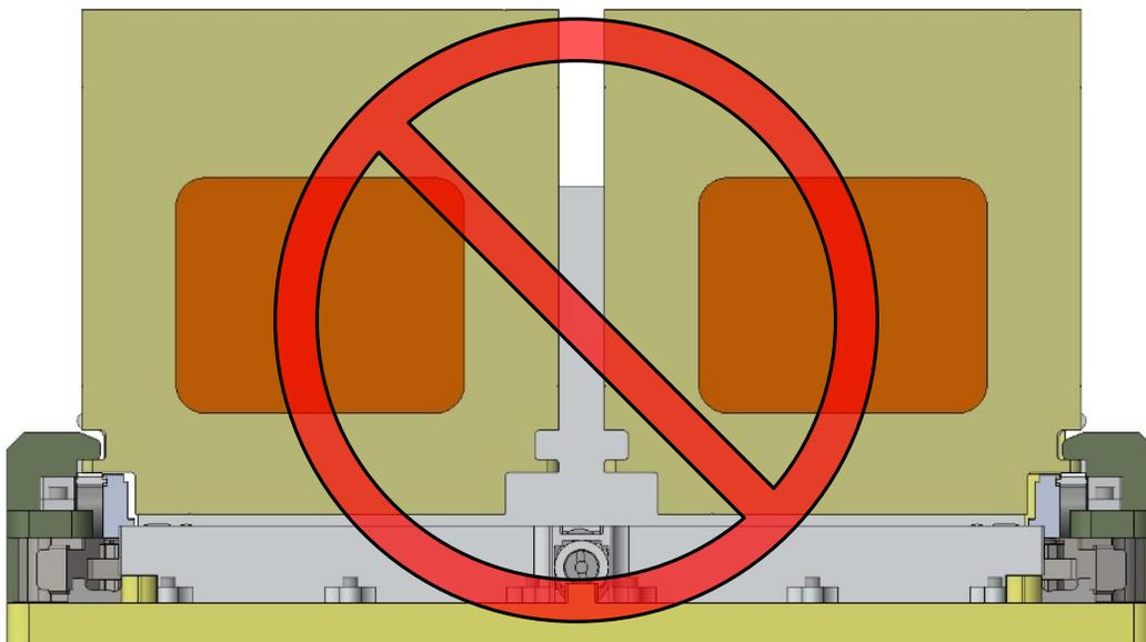
Figure 5-2: Two 3U payloads cannot be installed in an ASD
