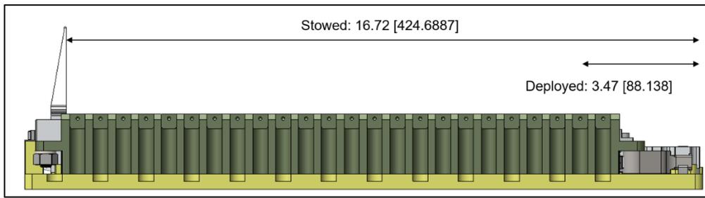
Figure 10-2: Ejection Plate travel
