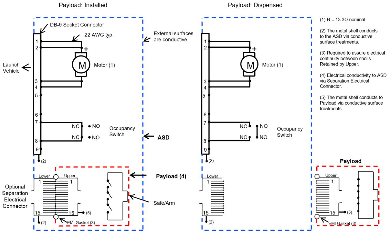
Figure 7-1: ASD electrical schematic
