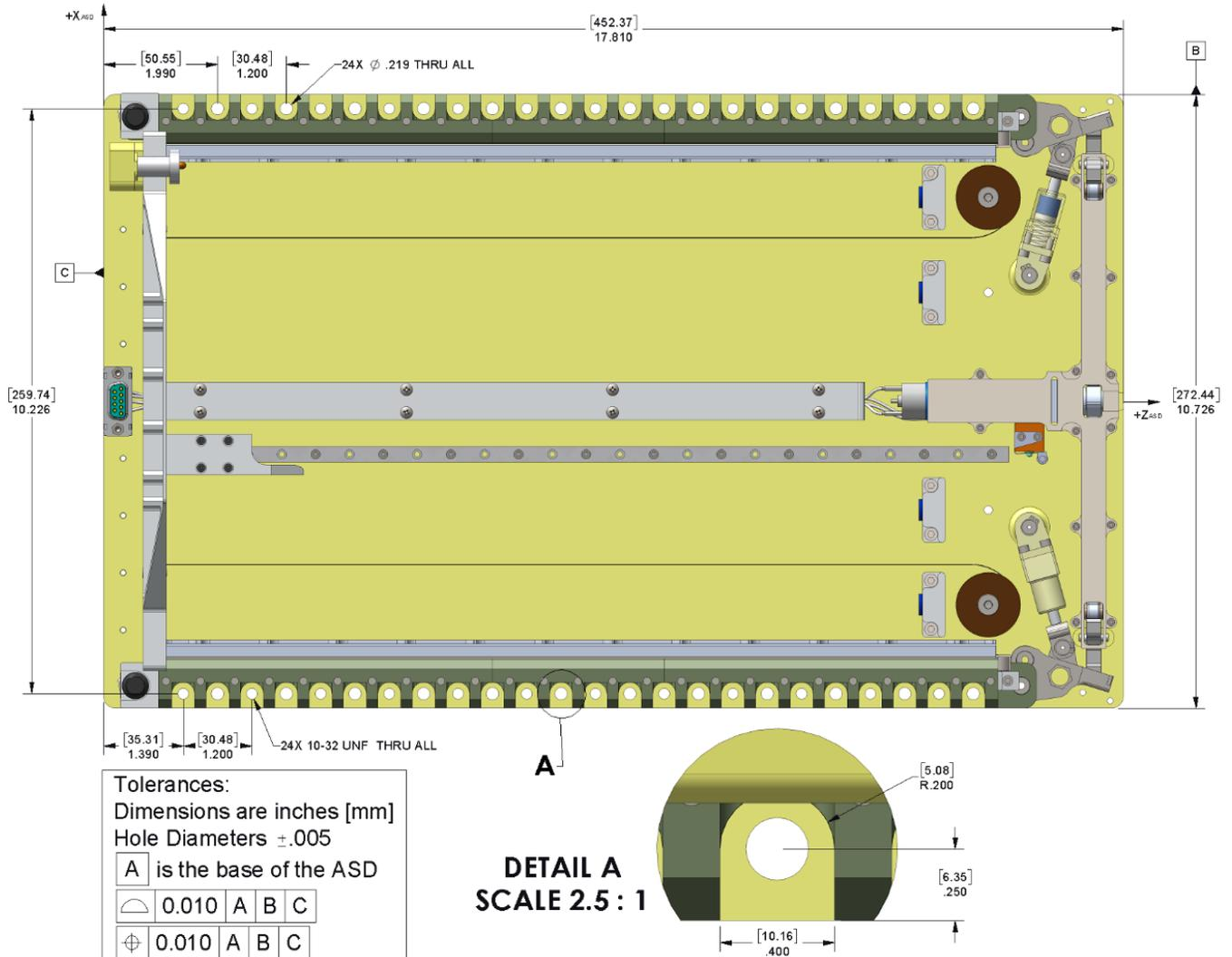
Figure 4-1: ASD mechanical interface dimensions
