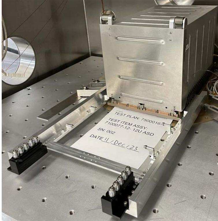
Figure 16-1: ASD with conveyor in TVAC
