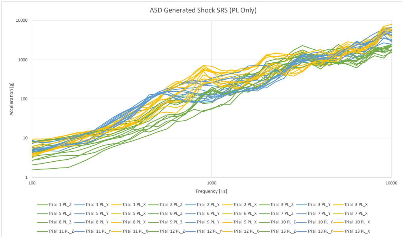
Figure 9-8: Shock measured on the payload
