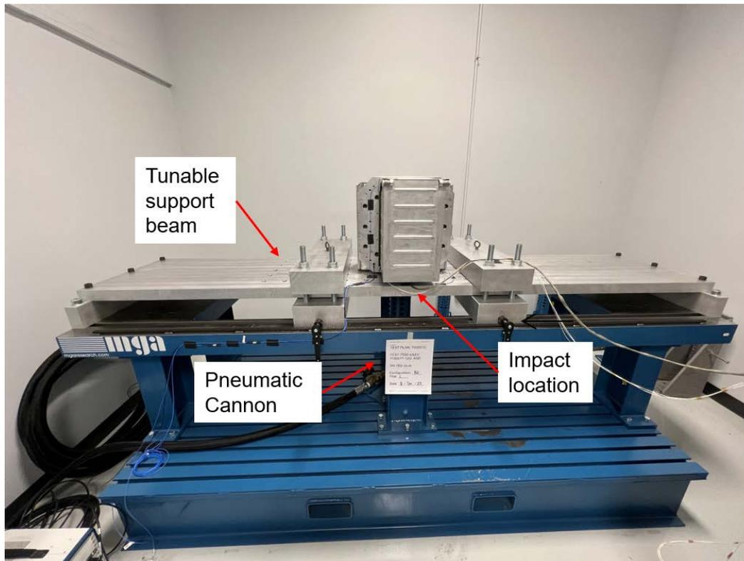
Figure 9-5: PSC-RL's shock test fixture
