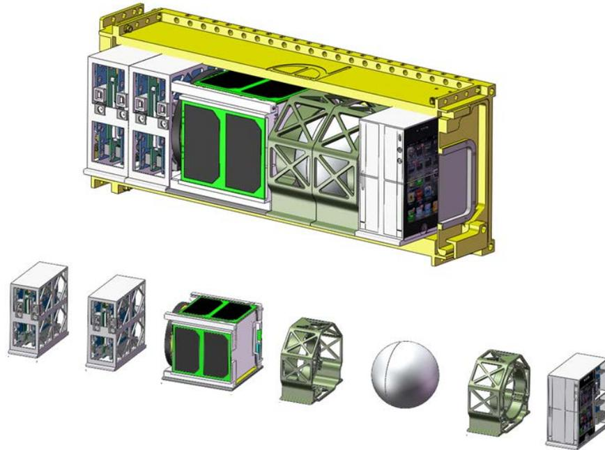
Figure 15-5: Multiple payloads in a CSD (also applies to ASD)
