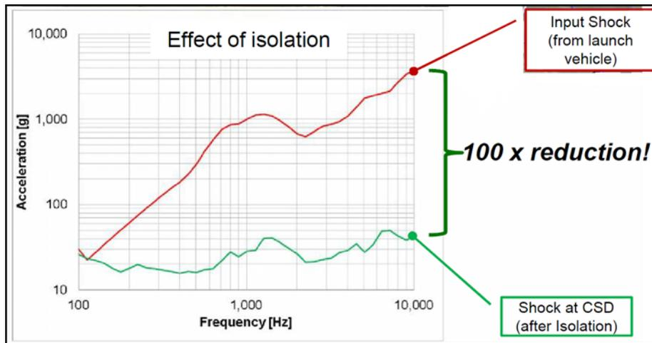
Figure 14-3: Isolation benefits during shock testing
