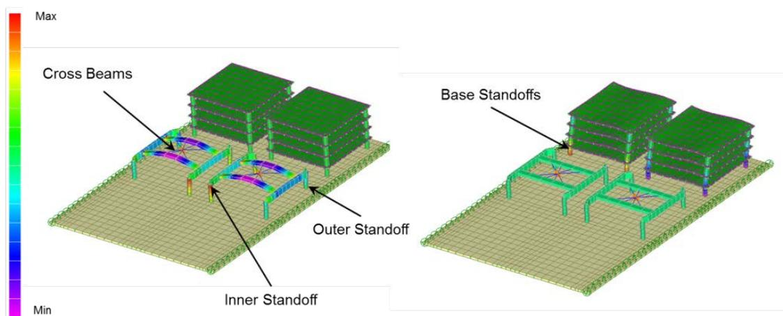
Figure 2-5: Identifying components with high strain
