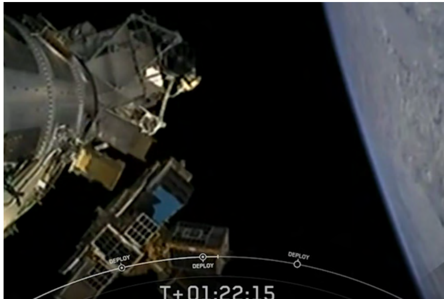
Figure 1-3: Two ALB 24 Separate FX-2 and LTE-1 from SpaceX's Transporter-2 using ALB 24
