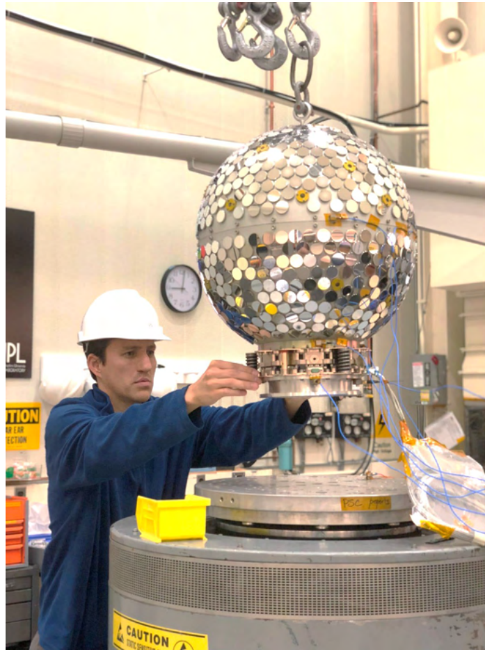
Figure 1-2: An ALB attached to Starshine-4 during a pre-flight vibration test
