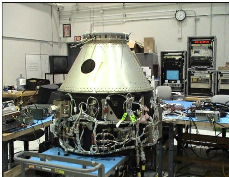
Figure 10-1: Electro-mechanical fit check and a separation test
