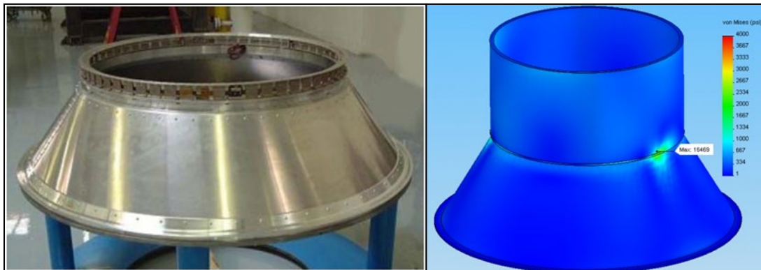
Figure 3-11: An MLB attached to a launch vehicle cone and CAD model showing resulting stress peaking that occurs when adjoining two warped surfaces
