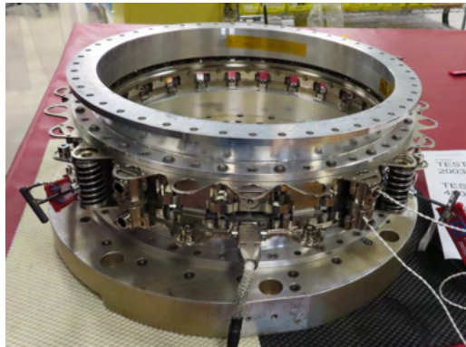
Figure 6-1: Benchtop Separation Testing
