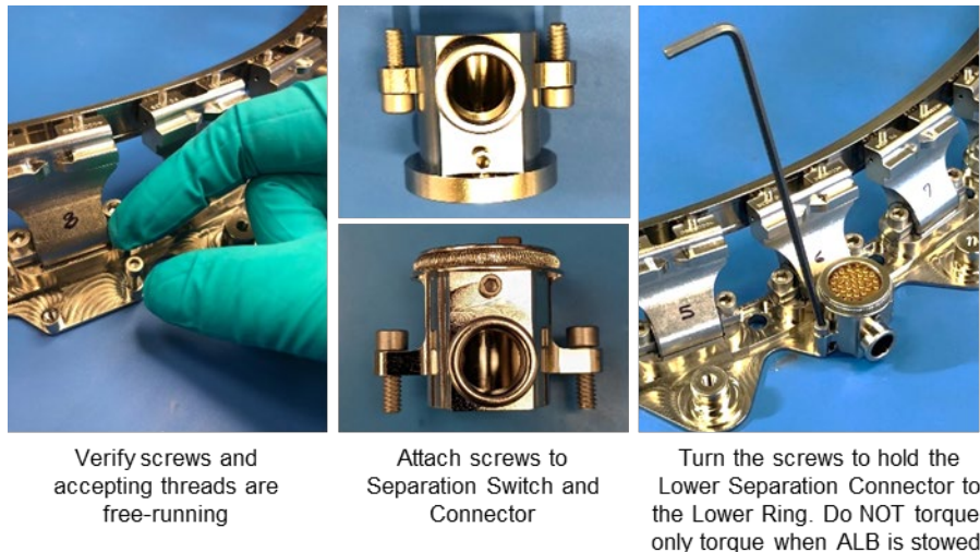
Figure 4-15: Attaching Separation Connectors
