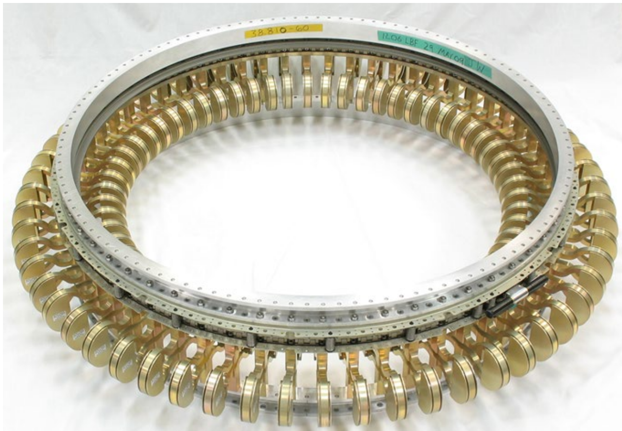
Figure 3-14: Moog CSA's SoftRide OmniFlex which isolates the satellite from the launch vehicle loads
