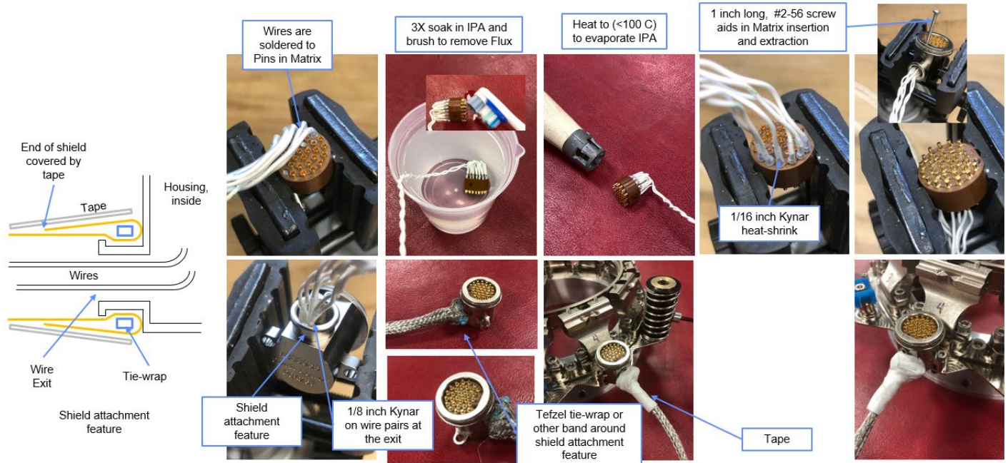
Figure 15-5: Wiring of Separation Connector
