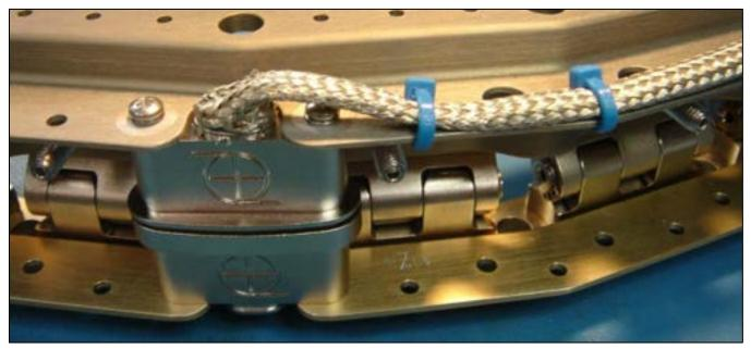
Figure 8-4: Through-holes on the outer lip of the MLB Upper and Lower Ring exist for routing tie wraps to support harnesses
