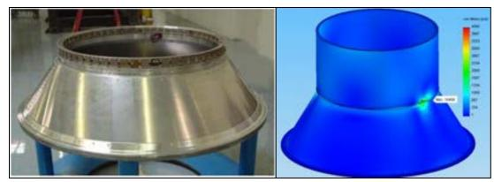
Figure 7-23: An MLB attached to a launch vehicle cone and CAD model showing resulting stress peaking that occurs when adjoining two warped surfaces
