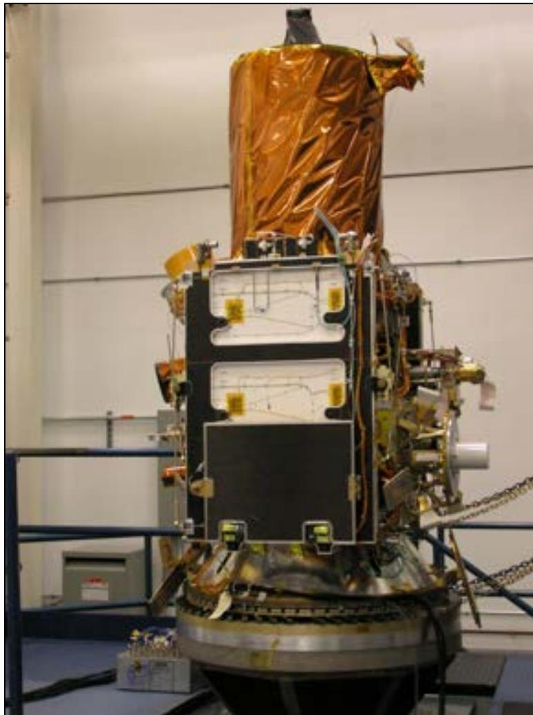
Figure 4-1: An MLB installed on the TacSat-2 mission
