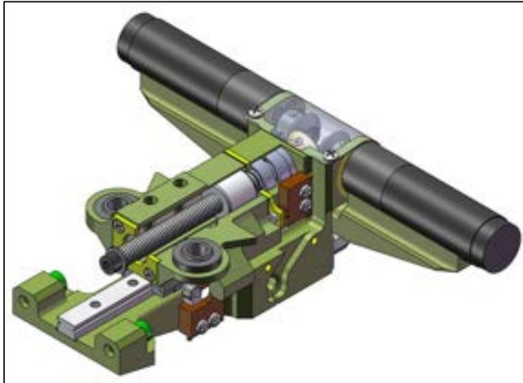
**Figure 7-13: Motor Bracket Assembly in the stowed state**
