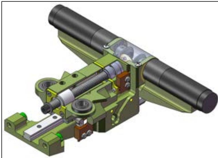
**Figure 7-14: Motor Bracket Assembly in the set-for-flight state**
