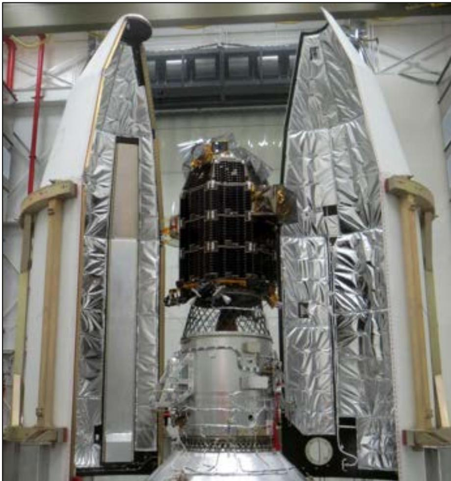
Figure 2-8: Two MLBs installed on a lunar payload prior to launch<sup>1</sup>
