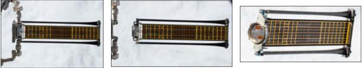
**Figure 14-1: 23 inch MLB deploying ROSA from ISS**
