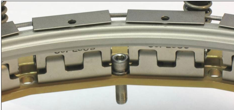
Figure 7-3: SHC screw and washer inserted between Leaves on elevated Lower Ring.
