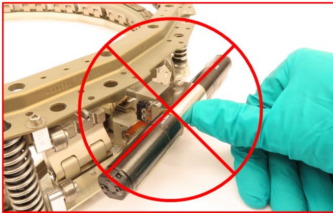
Figure 6-4: Do not touch the gear cover
