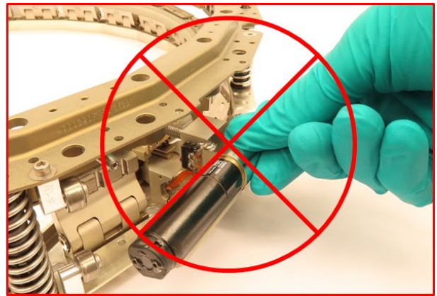
Figure 6-4: Do not touch the gear cover
