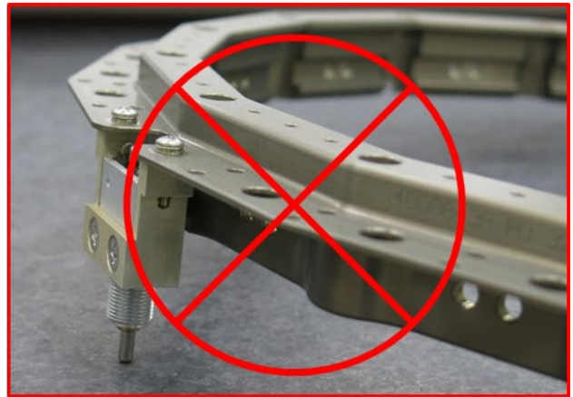
Figure 6-8: Do not allow Upper Ring accessories to contact anything
