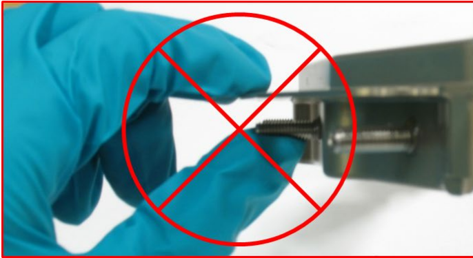
Figure 6-7: Do not touch spring plungers or allow them to contact anything
