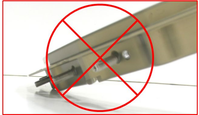
Figure 6-7: Do not touch spring plungers or allow them to contact anything
