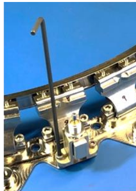
Turn the screws to hold the Separation Switch to the Upper or Lower Ring
