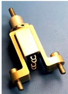
Attach screws to Separation Switch
