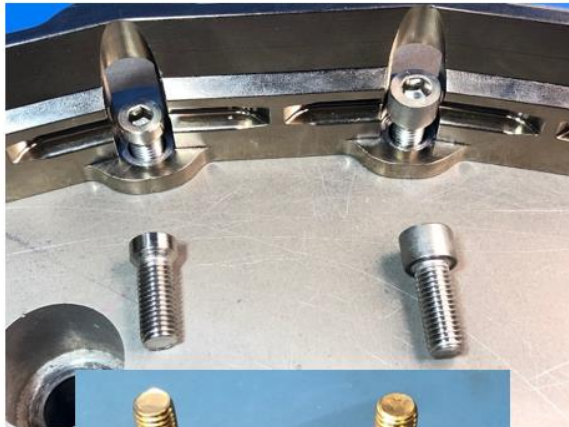
Figure 9-2: Fasteners and torques for adjoining structures
