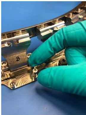
Verify screws and accepting threads are free-running
