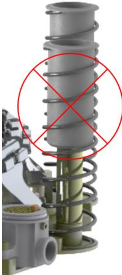
Figure 7-4: Do not use Springs to rotate ALB
