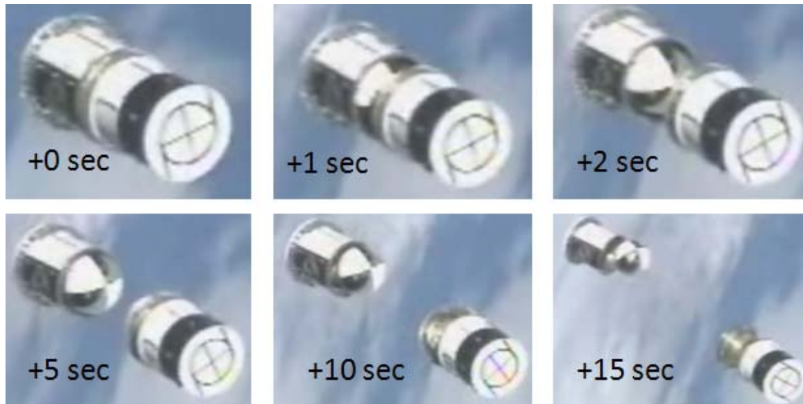
Figure 8. Actual On-Orbit ICU Separation Event
