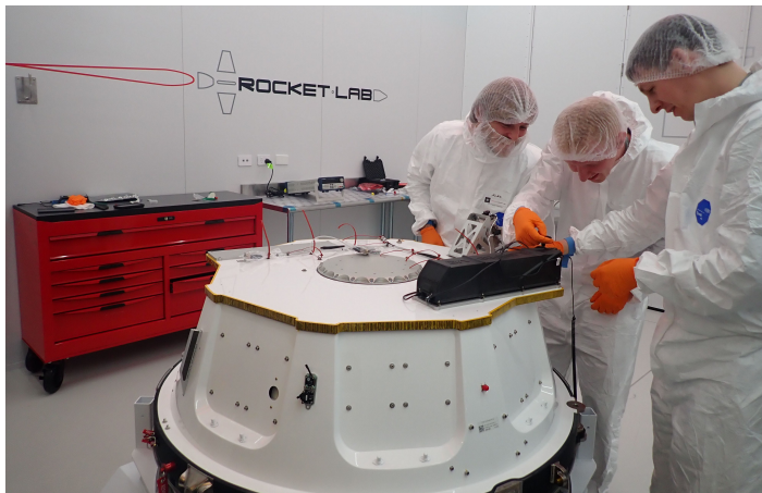
ALBA ORBITAL INTEGRATING THEIR ALBAPOD TO ELECTRON'S KICK STAGE AT LAUNCH COMPLEX 1 | November 2019
