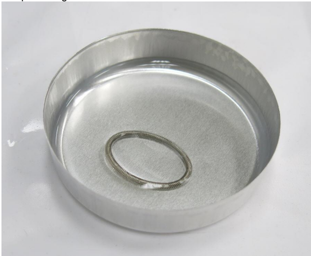
Figure 22: EMI gasket in clean IPA bath
