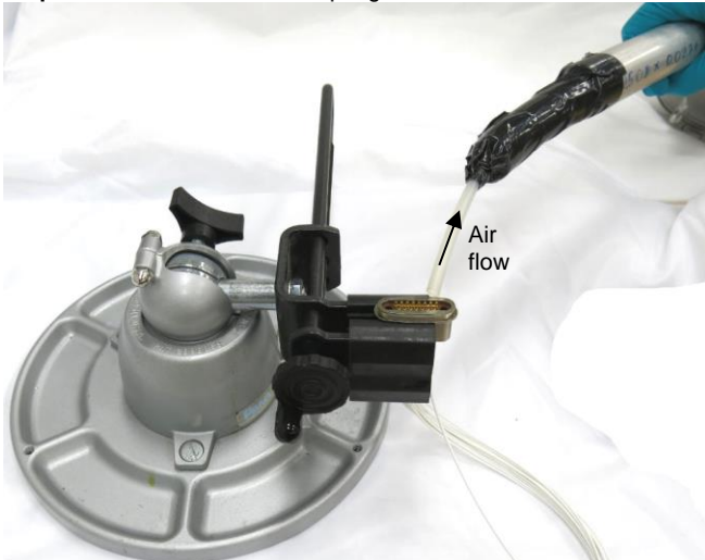
Figure 26: Vacuuming connector spring contacts with custom vacuum attachment
