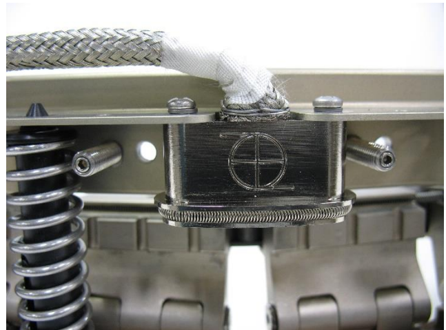
Figure 18: Upper Connector installed on Upper Ring. Harness is taped and formed.
