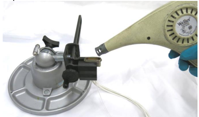
Figure 29: Heating the connector back shell to evaporate any remaining IPA
