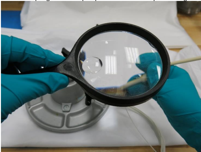
Figure 27: Use clean blunt edged plastic pick to compress spring contacts
