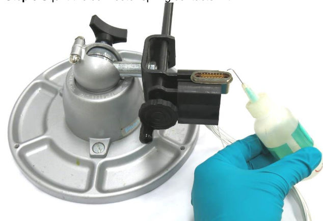
Figure 24: Squinting the spring contacts with IPA
